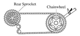
Each time the chain passes over one tooth on the chainwheel, it also passes over one tooth on the rear sprocket. Therefore, the rear sprocket will go through three revolutions for every one revolution of the chainwheel.
